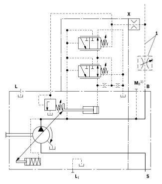
1 The metering orifice and the pressure relief valve and line are not included in the scope of delivery.
