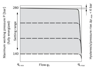
Characteristic curves valid at  $n_1$  = 1500 rpm and  $\theta_{fluid}$  = 50 °C. Control fluid consumption: 3 to 4.5 l/min. Standby standard 14 bar. Other values on request.
