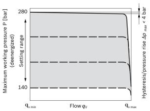
Characteristic curves valid at  $n_1$  = 1500 rpm and  $\theta_{fluid}$  = 50 °C. Control fluid consumption: 3 to 4.5 l/min.
