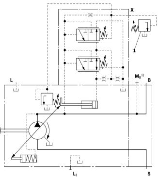
▼ Circuit diagram LA.S with separate flow control
