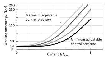
Hysteresis static current-pressure characteristic curve < 3 bar.
