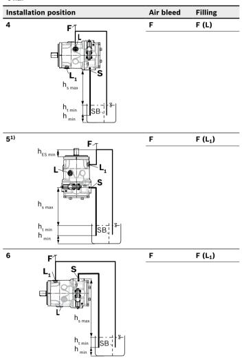
A check valve in the drain line is only permissible in individual cases. Consult us for approval.
