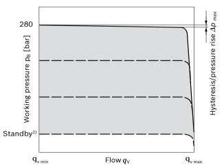
Characteristic curve valid for  $n_1$  = 1500 rpm and  $\theta_{fluid}$  = 50 °C.
