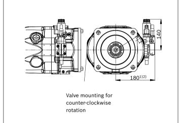
$<sup>\</sup>scriptstyle{\mbox{\scriptsize 1)}}$  ER7. 215 mm if using an intermediate plate pressure controller
