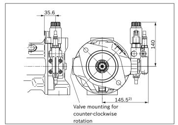
$_{\mbox{\scriptsize 1)}}\,$  ER7. 180.5 mm if using an intermediate plate pressure controller
