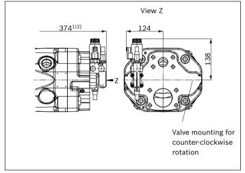
$_{\mbox{\scriptsize 1)}}\,$  ER7. 409 mm if using an intermediate plate pressure controller
