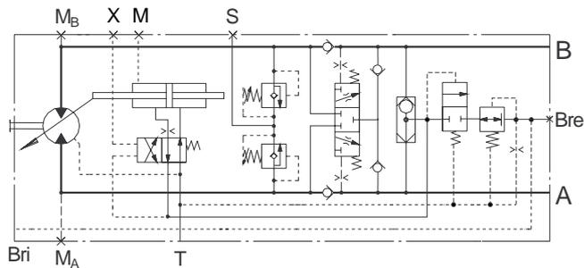
A6VE...HZ3...222 (brake release via external piping)
